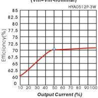
Efficiency VS Output Load curve (Vin=Vin-nominal)
