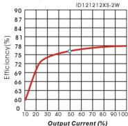
Efficiency VS Output Load curve (Vin=Vin-nominal)
